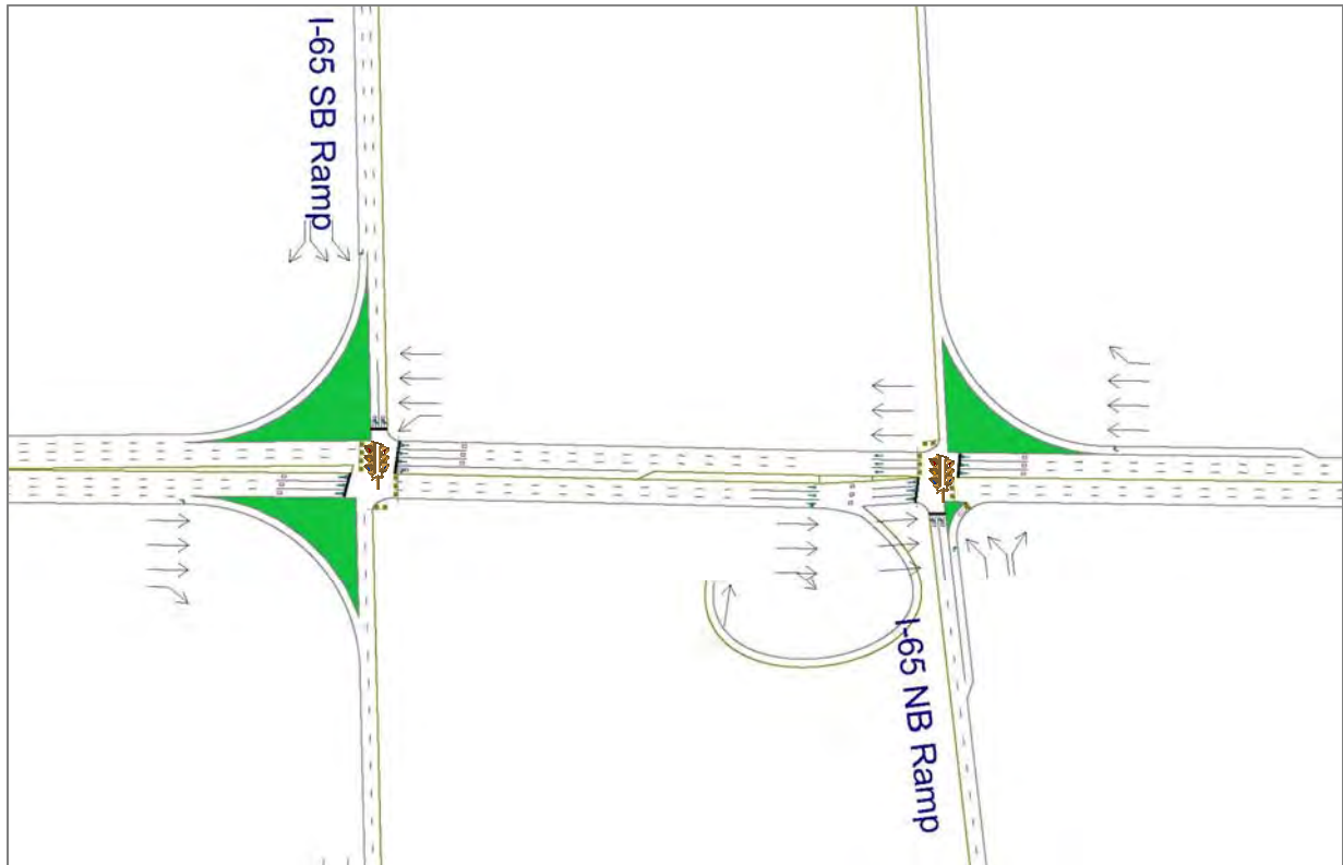
FIGURE 13- Partial Cloverleaf Interchange
